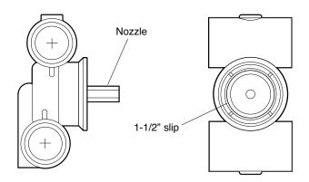
The jet body is available with a 1.5" slip socket that accepts standard 1.5" PVC pipe, providing maximum performance and flexibility for varying wall thicknesses.
